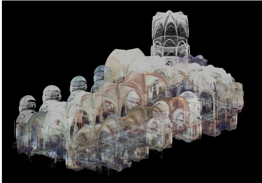
Fig. 3 - Point cloud model of the Cathedral's inner space
