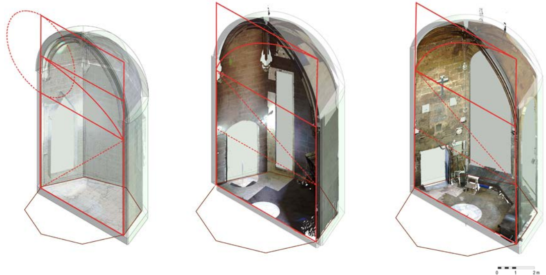
Fig. 9. The height of the vault is determined by the diagonal proportion in the first level and by the golden proportion in the second and third levels.
