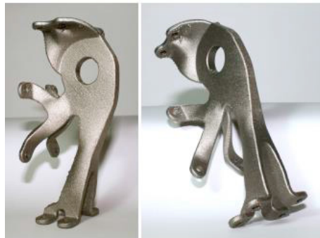
Fig. 8 – Optimised component manufactured.
