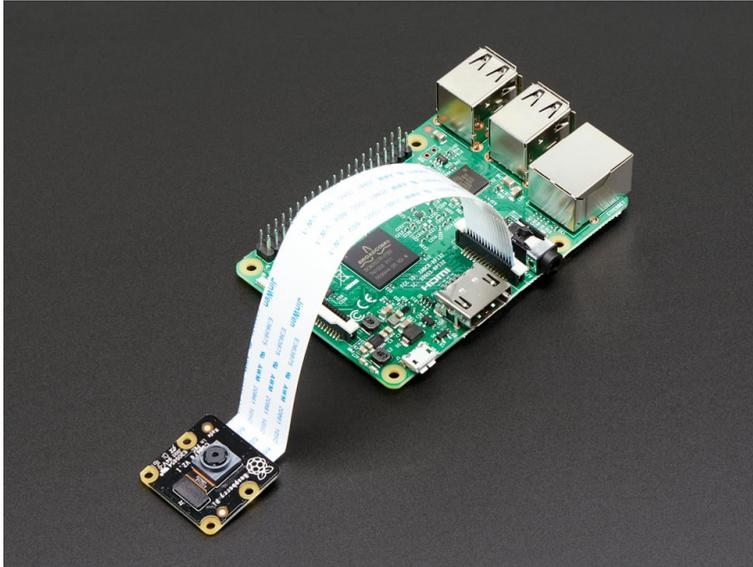
Figura 3.4: Cámara Raspberry Pi NoIR Camera V2 [66].
