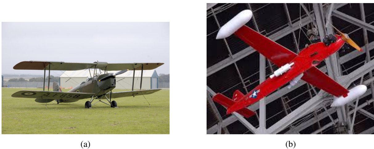
Figure 1.2: After war drones: (a) The DH.82B Queen Bee drone. (b) The SD-1, also known as the MQM-57 Falconer [1].
