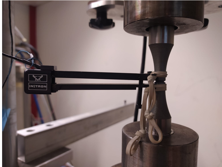
Figure 14: Extensometer setup for a A : 3 specimen.
