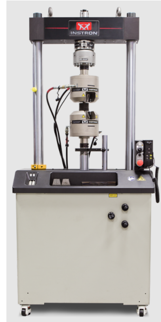
Figure 13: Generic servo hydraulic fatigue test rig 8801 [39].
