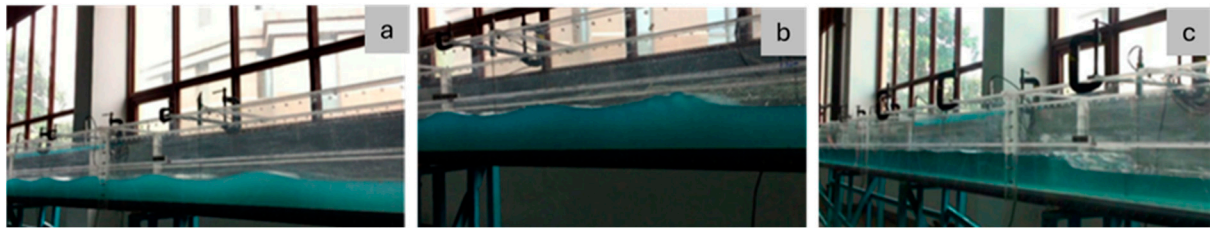
Figure 11. Tidal waves in different stages: (a) non-breaking undular tidal waves (stage 2), (b) breaking undular tidal waves (stage 3), and (c) breaking tidal waves (stage 4).
