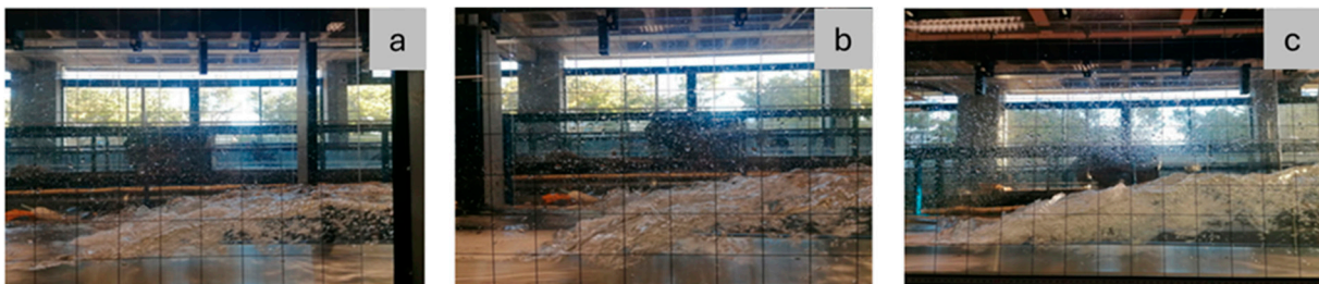
Figure 26. Hydraulic jump was observed during the laboratory tests for the same slope ( i = 0.1\% ), but different flow rates: (a) Q = 60 \text{ m}^3/\text{h} , (b) Q = 80 \text{ m}^3/\text{h} , and (c) Q = 100 \text{ m}^3/\text{h} .
