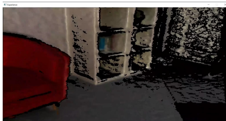
Figure 3. GUI of BundleFusion showing the reconstruction in real-time.
