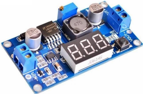
Figure 2: DFR0379 Adjustable DC to DC voltage regulator [10].
