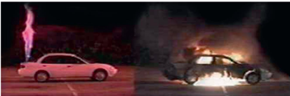
Figure 5: Demonstration of hydrogen safety: hydrogen fire (left) versus gasoline fire (right) [7]
