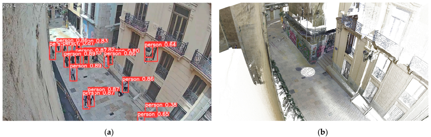
Figure 2. (a) Original camera view with person counting system. (b) Recreation of camera view using point cloud.
