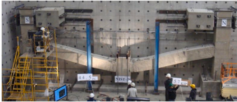
Fig. 19. Full-scale seismic detailed sub-assembly for column-removal testing [160].
