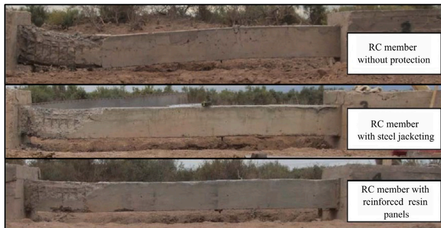
Fig. 18. Member retrofitting impact [106].
