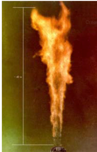
Figure 7.21: IVG-1: Startup, at 225 MW and outlet temperature of 3000 K. Source: Kurchatov Institute.
