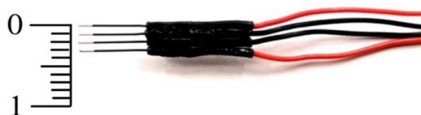
Figure 1. Arrangement of in-line, four-needle electrodes used to measure electrical impedance. The two outermost electrodes injected the electrical current, while the two central electrodes picked up the electrical voltage (scale in mm).
