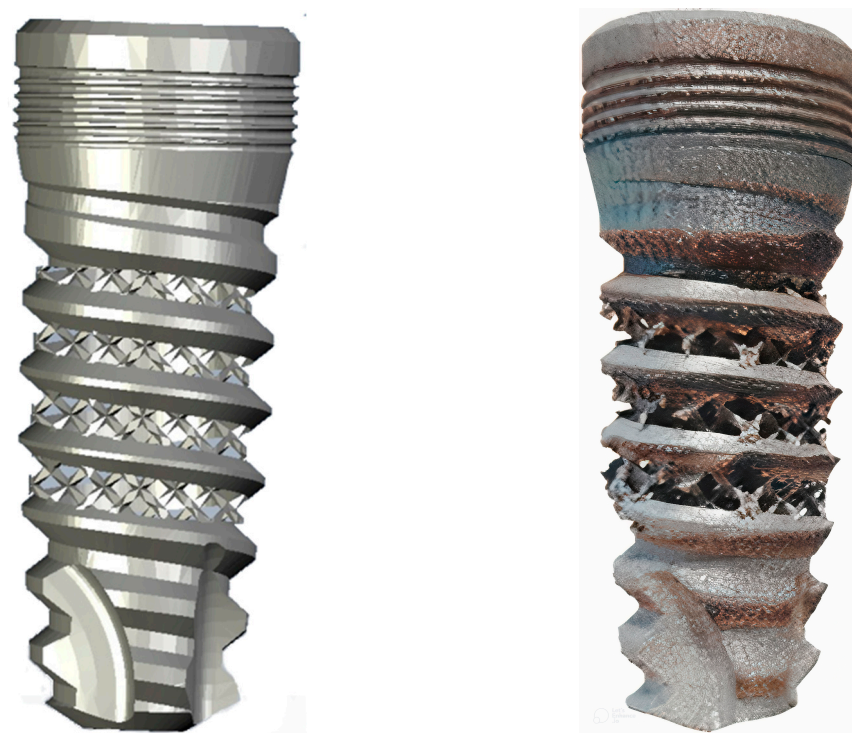
Figure 6. Implant body manufactured by additive 3D printing before machining its internal thread. Left side image, computer recreation. Right side the 3D printed implant.
