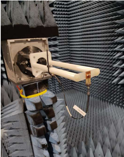
FIGURE 6. Measurement of the prototype in an anechoic chamber with the reference antenna technique.
