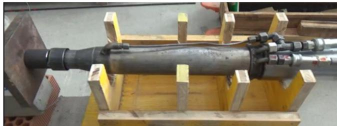
Fig. 9: Mono-strand jack for 15.2-mm strand diameter.
