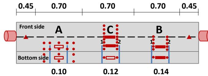
Fig. 3: Instrumentation layout of Beam 1.
