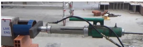
Fig. 5: Mono-strand jack for 13-mm strand diameter.
