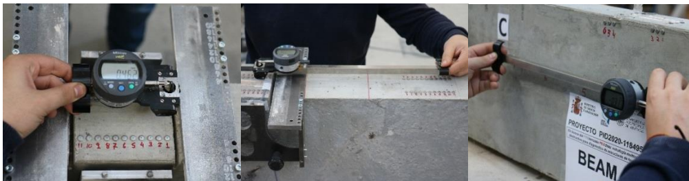
Figure 14. Measurements using DEMECs, Measurement base 100 and 400 MILLimeters
