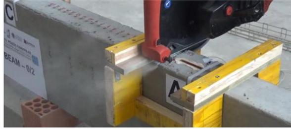
Fig. 7: Performing a saw cut in Beam 2a.
