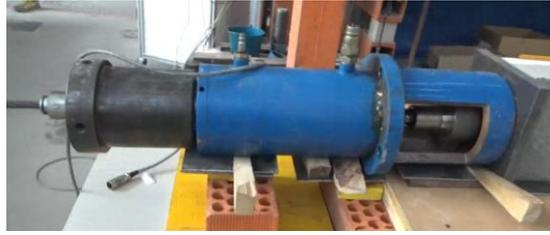
Fig. 2: Hollow hydraulic jack with and adjustable mechanical anchorage.
