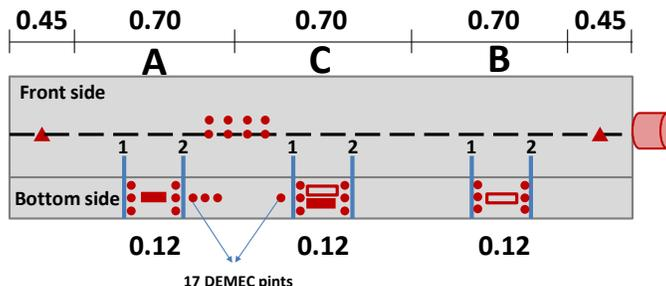
Fig. 6: Instrumentation layout of Beam 2a.
