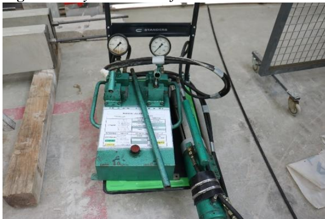
Figure 12. Hydraulic Jack for Prestress
