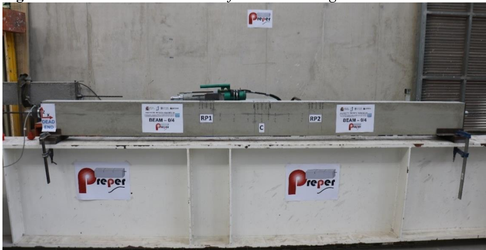
Figure 15. SPCE in its Final State Before Detensioning
