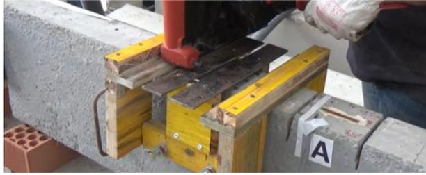
Fig. 10: Performing a saw cut in Beam 2b.
