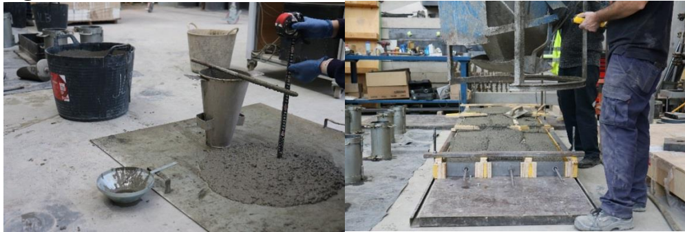
Figure 10. Abrams Cone and Placement in the Concrete Formwork
