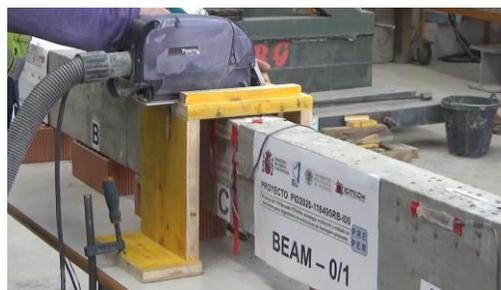
Fig. 4: Performing a saw cut in Beam 1.
