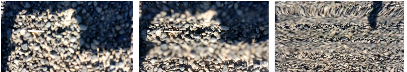
Figure 5.10: The images from left to right show the camera image evolution when propellers start spinning during a takeoff.
