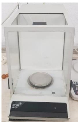
Figura 40. Balanza Metler Toledo AE240.
