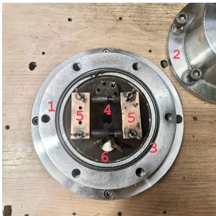
Figure 3.3: Close view from above of a wire mesh reactor
