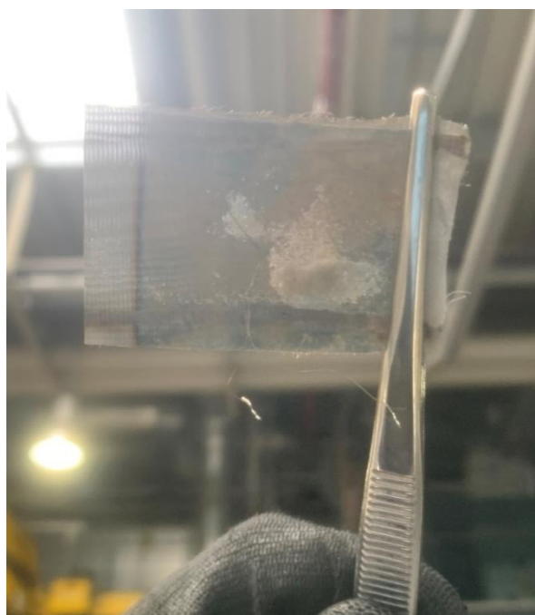
Figure 3.7: Net filled up with polystyrene sample
