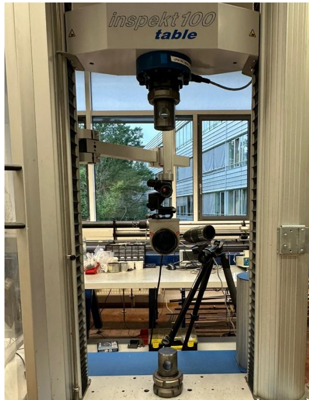
Figure 3-5: Static electromechanical universal testing machine (Hegewald & Peschke – Inspekt)
