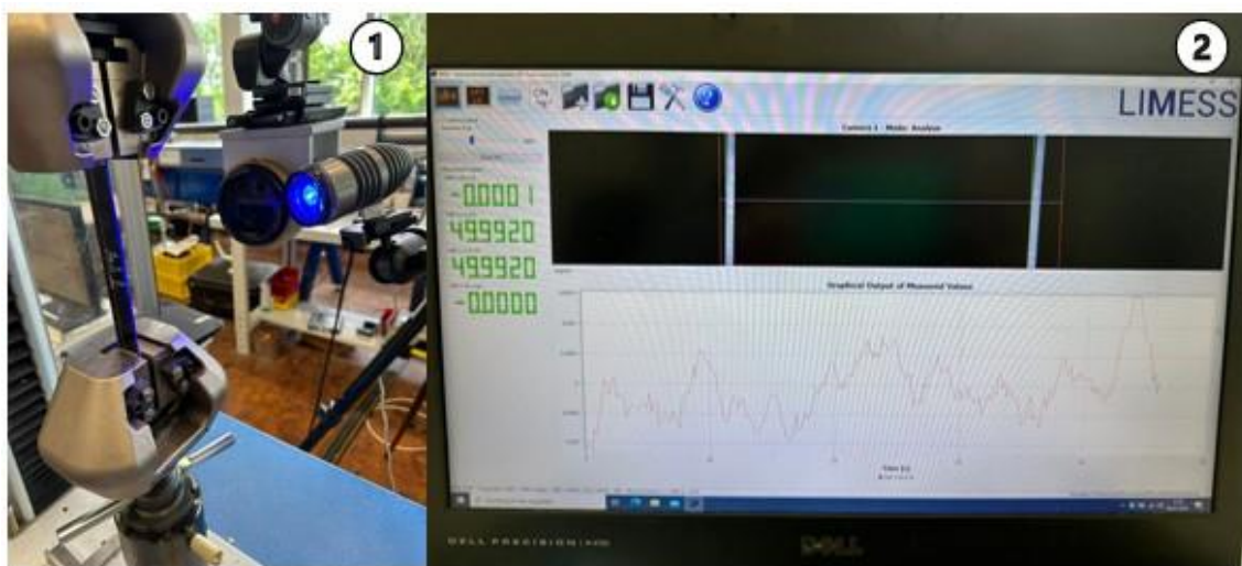
Figure 3-6: 1) Video extensometer, and 2) the respective software
