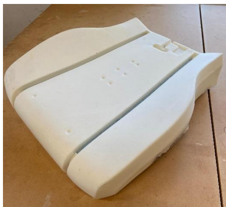
Figure 14. Foam bolster structure.
