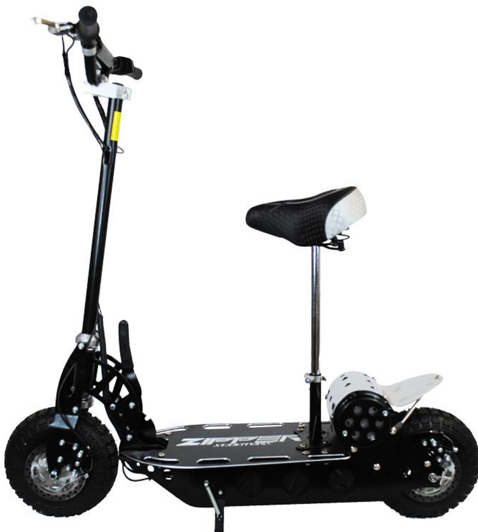
Figure 29. Electric kickboard with a motor mounted outside the rear wheel(obtained from scootercity.co.uk )
