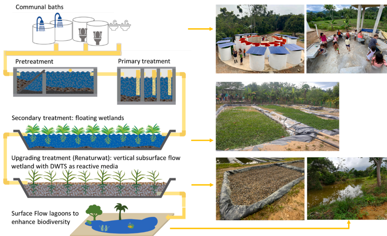
Fig. 1. Scheme of the sanitation system projected and built in Embera Katío indigenous communities and pictures of the functional components.
