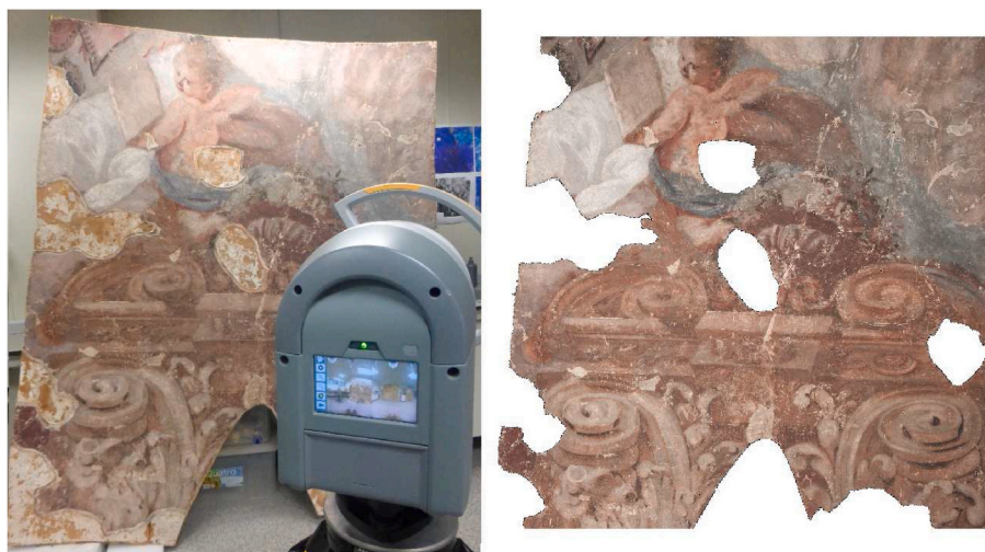
Fig. 3. Panel number 11 (a) Panel laser scanning (3D), (b) Panel orthophotography (2D).
