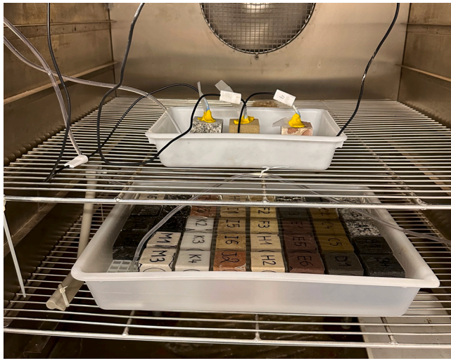
Fig. 3. Monitoring of temperatures in independent samples at the top and saturation tray at the bottom.
