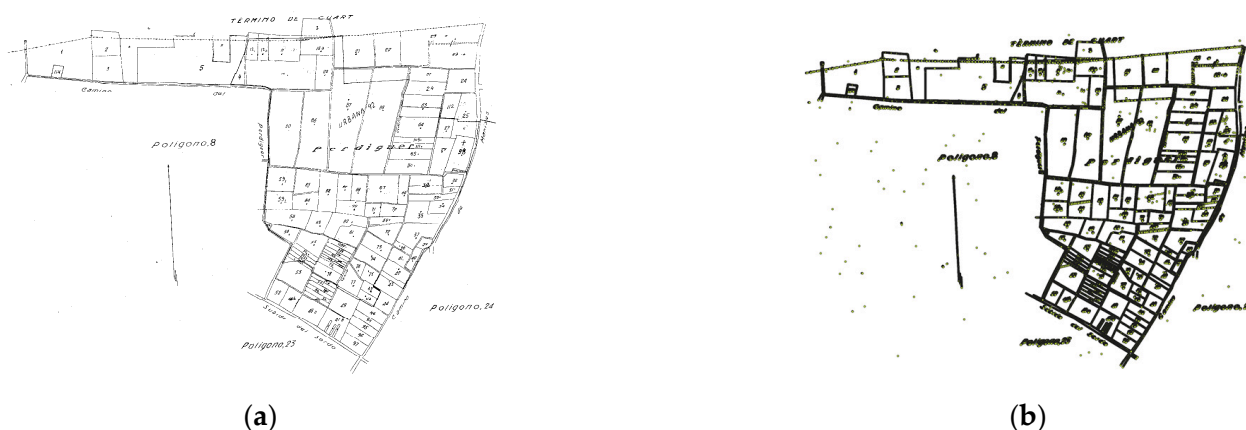
Figure 10. OCM process to obtain the cadastral polygon perimeter. Steps one and two: (a) frame cleaning by applying a mask; (b) deriving vector points from the raster pixels. Source: Authors.
