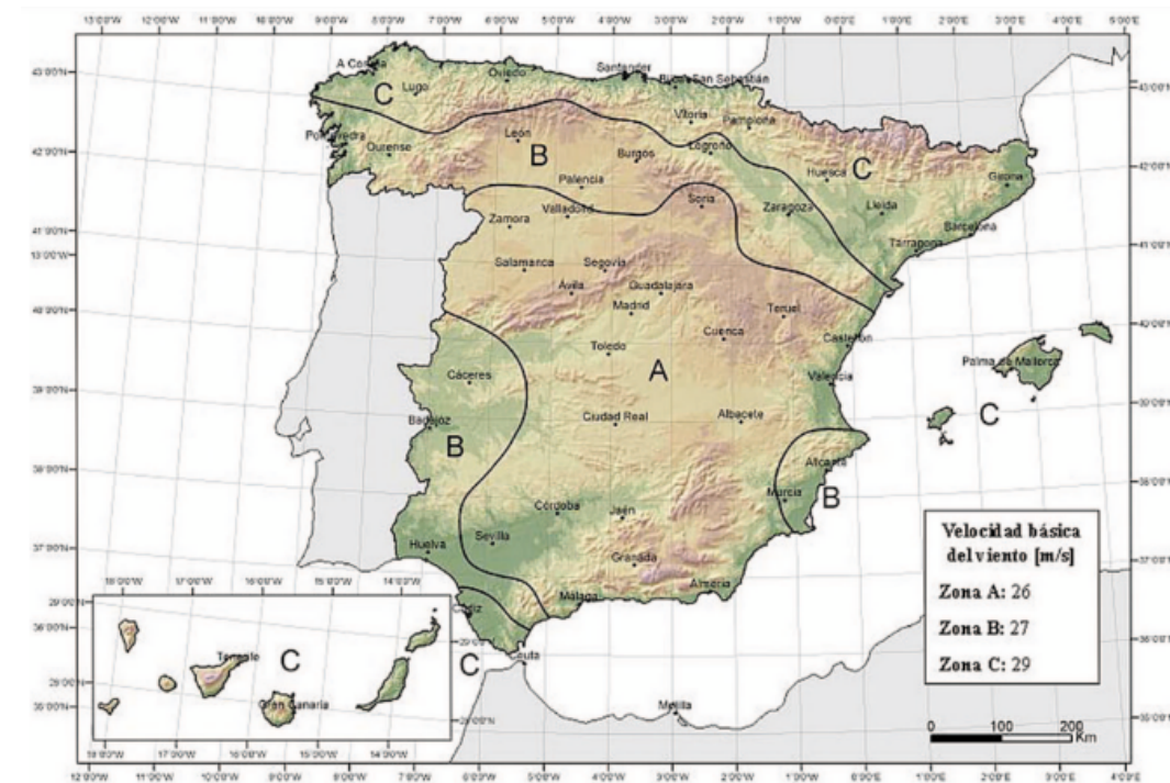
Figure 6: Isotach map for obtaining the basic fundamental wind speed v_{b,0} [IAP-11]
