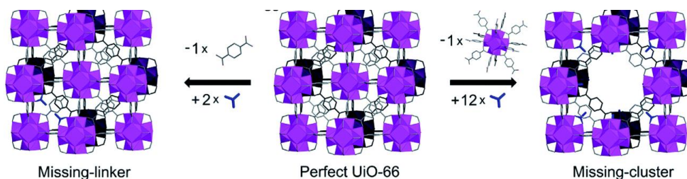
Figure 17. Structural UiO-66 differences between the ideal unit cell and those with missing linker or missing cluster defects. Reproduced with permission from ref. 129 Copyright 2017, with permission from Elsevier.
