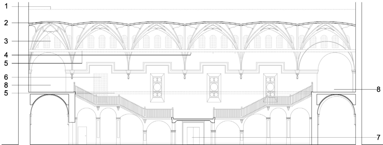
Legend: 1.- Key level of the medieval pointed arches. 2.- Partitioned vault. 3.- Blocked gallery of small arches. 4.- Remains of floor support. 5.- Level of the missing floor. 6.- Blocked window. 7.- Current access to the enclosure. 8.- Corridor leading to cells.
