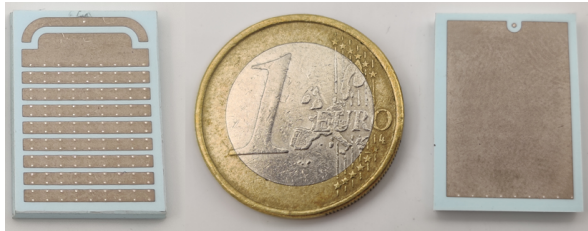
Figure 7.4: Front view of the fabricated LTCC 868 MHz on-ground chip antenna.
