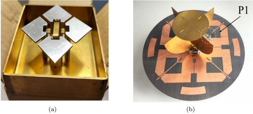
Figure 1.2: a) Picture of a compact wideband dual-polarized magnetolectric dipole antenna [13] and, b) Dual-polarized wideband omnidirectional ceiling antenna with low gain variations (GVs) [14].
