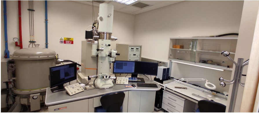
Figure 29. JEOL 2100F Transmission Electron Microscope (TEM) room situated at the Universitat Politècnica de València (UPV) microscope services. The operating voltage is set at 200 keV. The left section of the image showcases the high tension (HT) tank. The central portion displays the TEM, control panels, monitors, and the high vacuum system. The right section features the table used for grid preparation along with the Nanomegas precession device.
