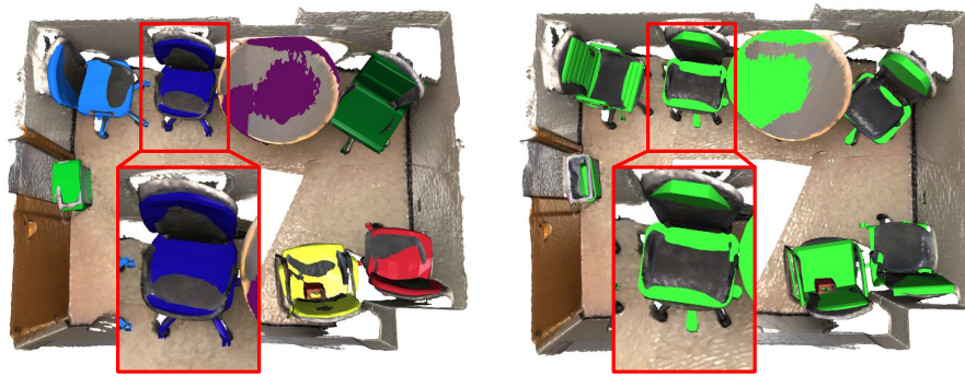
Fig. 6: Comparison between 2 CAD retrieval and alignment methods using a ScanNet validation scene. From left to right: ScanNotate and Scan2CAD results.
