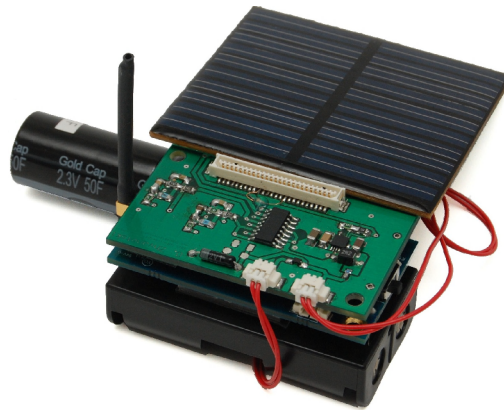
Figure 3.1: Energy Harvesting Platform for the Iris node [48]
