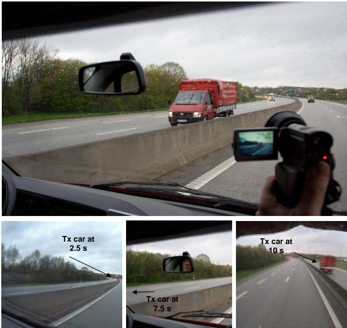
Fig. 24: General view of the scenario and screenshots from the video of the measurement run: The Rx car approaching the Tx car, The Rx car passing by the Tx car and The Rx driving away from the Tx car (From LEFT to RIGHT)
