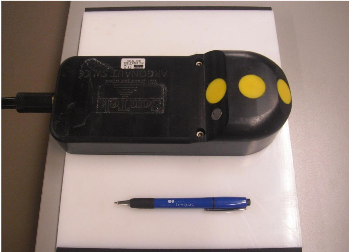
Figura 3.3 El ADCP Argonaut SW 3000 kHz
