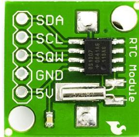
FIGURA 9.6: MÓDULO RTC (REAL TIME CLOCK) DE SPARKFUN
