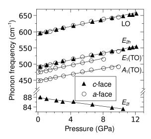
FIG. 3. Pressure dependence of the optical phonon frequencies of w-InN measured in the upstroke in c-face InN (solid triangles) and in the a-face InN (open circles). The lines are the results of linear fits to the experimental data.
