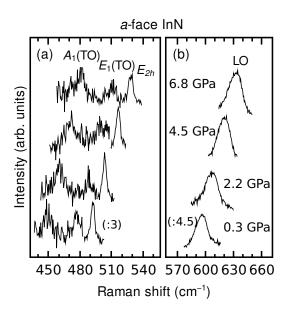
FIG. 2. Room-temperature Raman spectra of a a-face InN layer at different hydrostatic pressures in the up-stroke (a) in the middle-frequency region and (b) in the high-frequency region.
