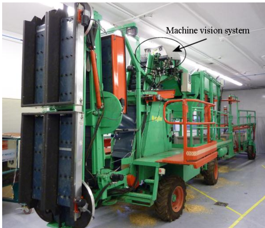
FIGURE 3. Mobile platform for citrus fruits harvesting
