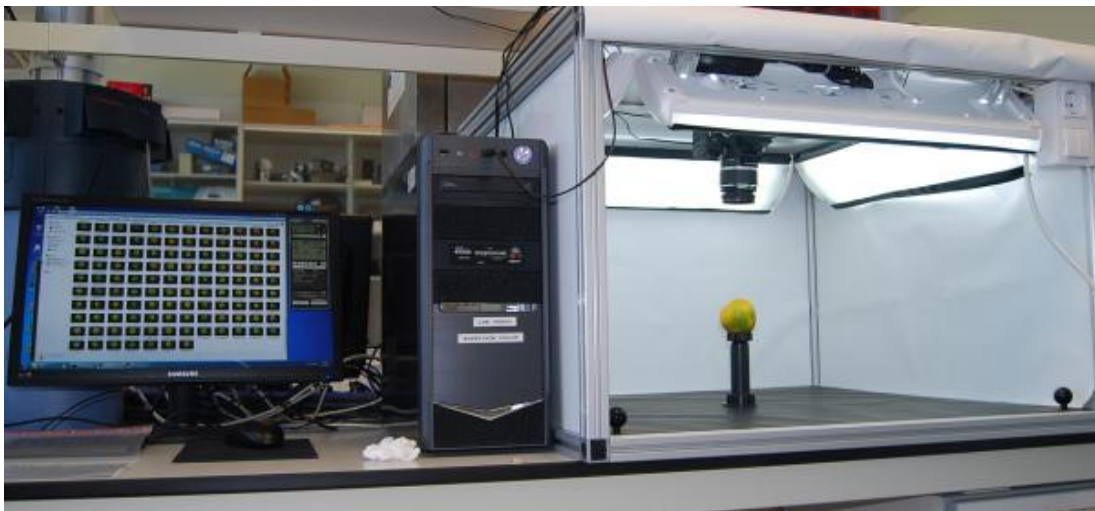
FIGURE 2. Inspection chamber used to capture high resolution images
