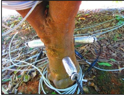
Figure 10 Distribution of the sensors installed in ‘Clementina de Nules’ trees.
