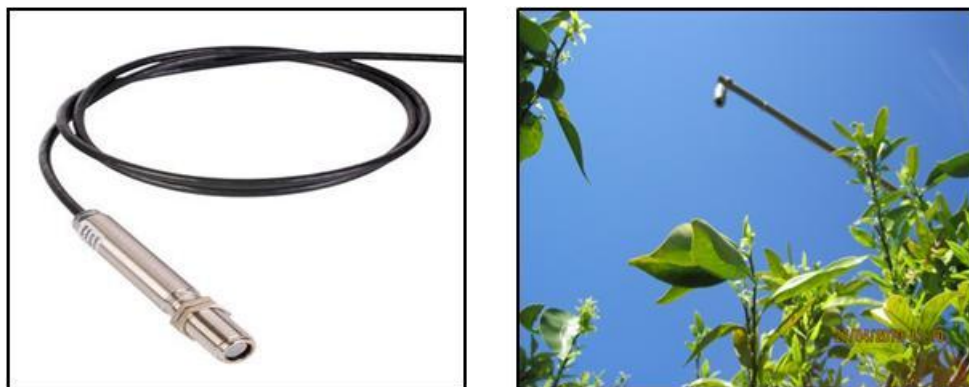
Figure 11 Infrared thermometer sensor employed in the ‘Clementina de Nules’ grove for the canopy temperature measurements.
