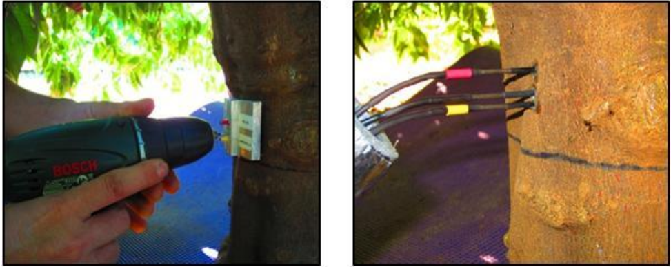
Figure 7 Installation of the sap flow sensors employed in ‘Navel Lane Late’ trees.
