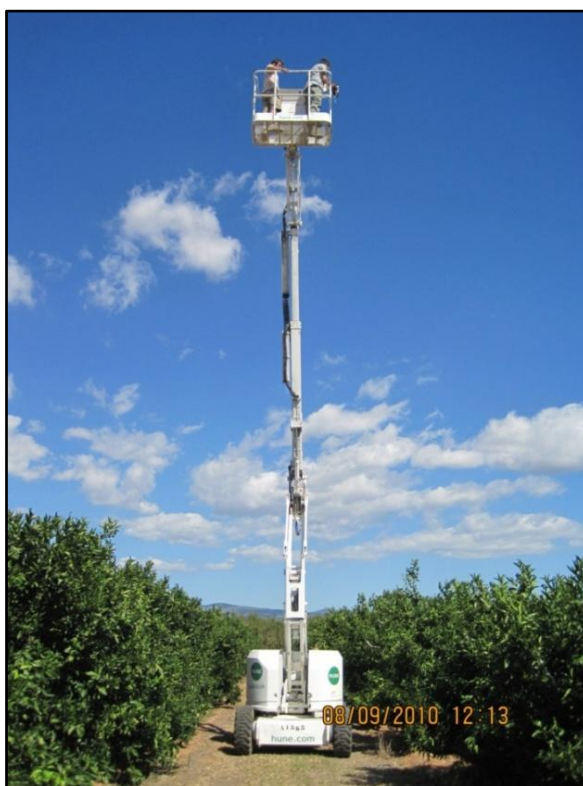
Figure 9 Truck-crane employed for the canopy temperature measurements.
