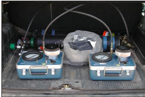
Figure 3 Cylinders and pressure chambers used for the stem water potential measurement.
