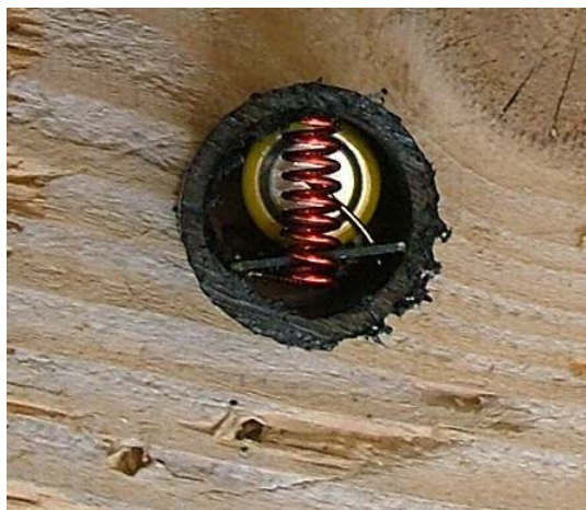
Figure 1. Node inserted in wood.
