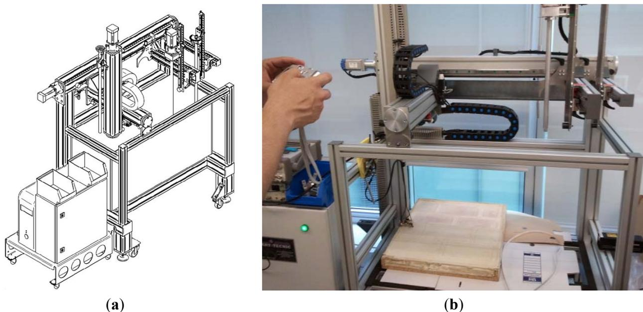
The surface measured covers  $25.5 \times 41.4 \text{ cm}^2$  in steps of 3 mm in both Cartesian axes X and Y. Thus, one measurement comprises  $138 \times 85$  mesh points, which corresponds to 11,730 measurement positions. The same XY measure was performed at two different heights. The sensor reference line was established at two different heights, 1 and 2 mm, measured from the lower part of our system to the test specimen surface marked as “h” in Figure 1.
