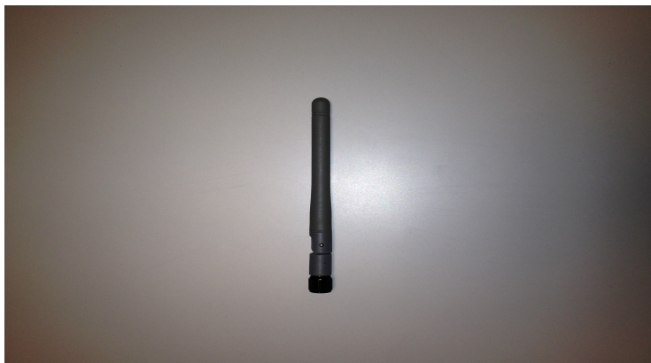
Figure (2.4.1): Short dipole.
