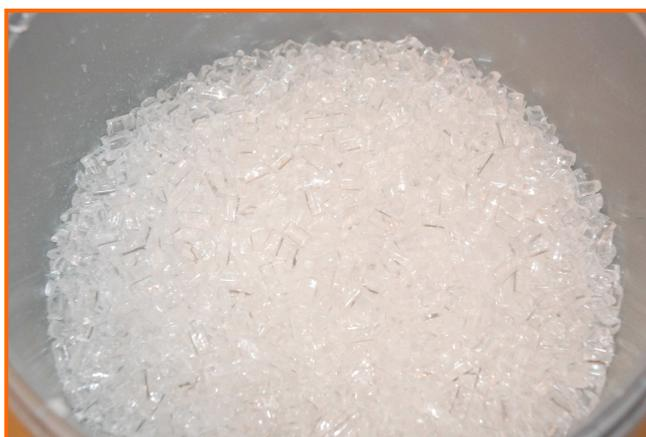
FIGURA 14. DETALLE RESINA PARALOD B-72
