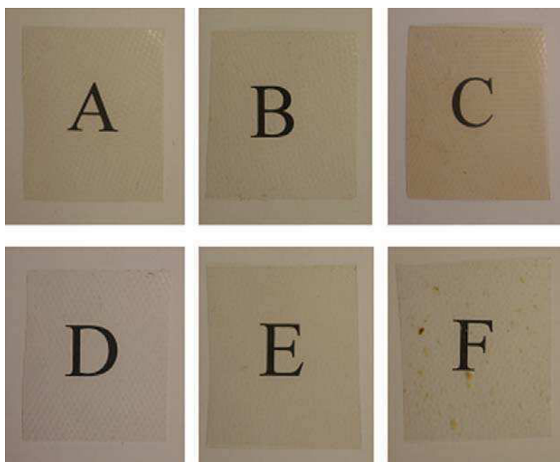
Figure 7. Photographs of films containing: (A) Pure EVOH; (B) EVOH+2 wt.-% BCNW precipitated; (C) EVOH+4 wt.-% BCNW precipitated; (D) EVOH+2 wt.-% BCNW ES; (E) EVOH+2 wt.-% BCNW freeze-dried/precipitated and (F) EVOH+2 wt.-% BCNW freeze-dried.
