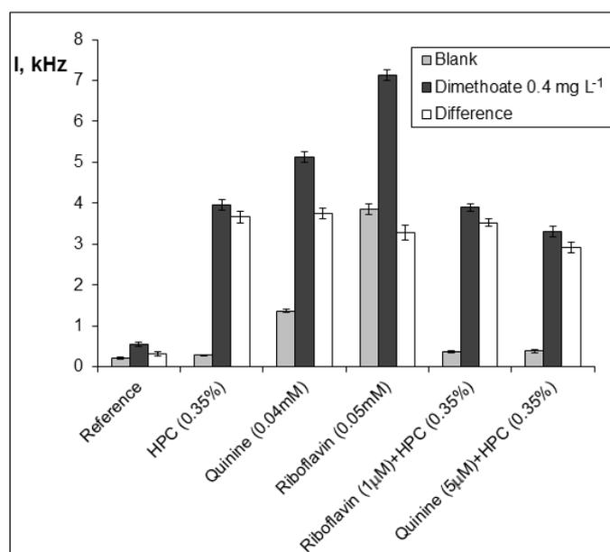
**Figure 3.** Effect of some sensitizers on the PICL of dimethoate 0.4 mg L<sup>-1</sup>. HPC: hexadecylpyridinium chloride; Uncertainty ( $\pm 2SD$ ) is indicated by error bars.
