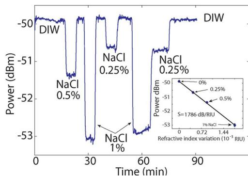
Fig. 5. (Color online) Time evolution of the output power during the flow of NaCl dilutions with different concentrations. The inset shows the sensitivity curve.
