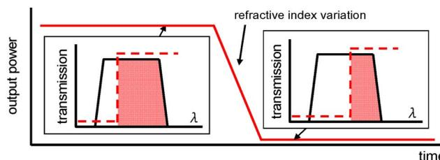
Fig. 1. (Color online) Output power evolution using the proposed sensing technique. In the initial state, the source spectrum (black solid line) is filtered by the PBG of the sensing structure (red dashed line) and only a certain amount of power is transmitted (shaded area). When a refractive index variation occurs, the PBG shifts, and the amount of input power filtered changes (decreases in this case).
