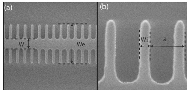
Fig. 3. (a) Scanning electron microscope image of the SOI corrugated waveguide used for sensing, (b) closeup view of the transversal elements.
