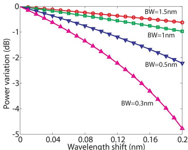
Fig. 2. (Color online) Power variation versus wavelength shift for different initial alignments between the source and the sensor. BW, initial overlapping bandwidth.
