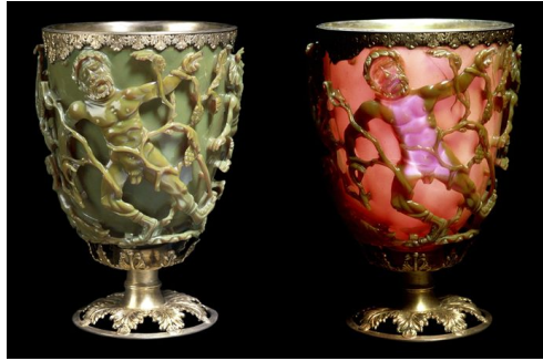
Figure 1.1: The Lygurus cup, probably made in Alexandria or Rome around 300AD, has embedded plasmonic nanoparticles in its glass. The glass appears green in reflected light and red in transmitted light.
