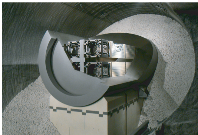
Figure 2.4. Storage model for nuclear spent fuel in the Grimsel Test Site in the Swiss Alps. Picture taken by the author of this manuscript during a NAGRA guided visit in the GTS.
