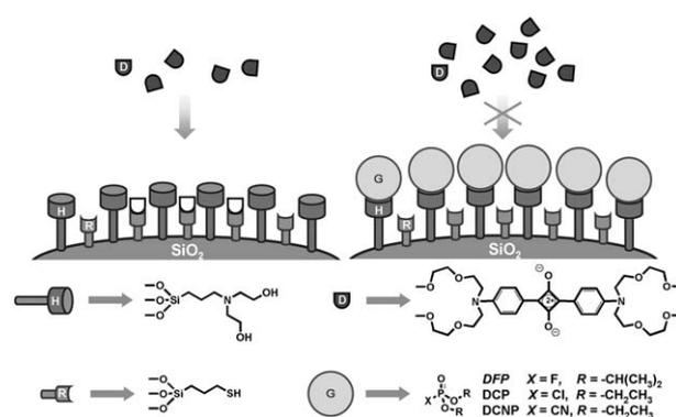
**Fig. 15** Analyte-mediated suppression of indicator decolouration.
