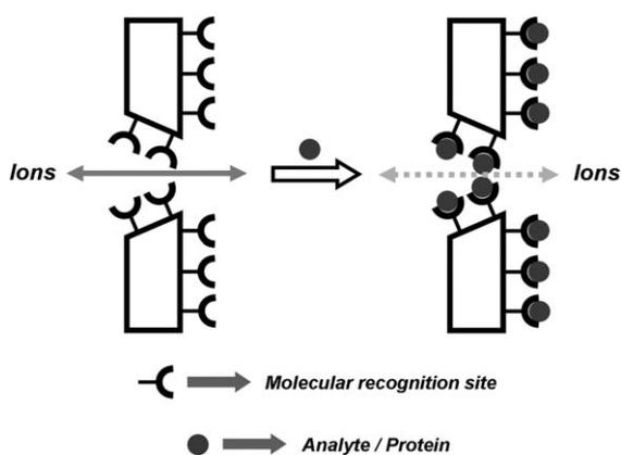
**Fig. 16** Architecture of a hybrid material containing a single nanopore and mode of operation by inhibition of ion flux.
