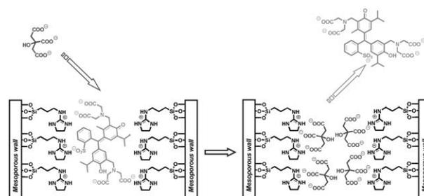
**Fig. 4** Protocol for citrate signalling in water by indicator displacement with a mesoporous solid containing guanidinium-functionalised nanoscopic binding pockets and methylthymol blue as the indicator.
