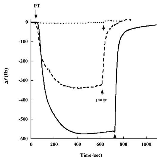
**Fig. 10** Frequency changes of QCM resonators coated with parathion-imprinted (solid line) and non-imprinted (dashed line) sol-gel films in response to parathion-saturated nitrogen. Upward arrow indicates the time of introduction of clean  $N_2$  stream into the chamber to desorb bound parathion. Dotted line: response of a bare, uncoated QCM resonator. (Reproduced with permission from ref. 59. Copyright American Chemical Society.)
