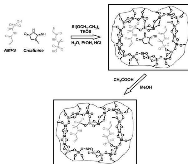
Fig. 8 Schematic preparation of the hybrid organic-inorganic sol-gel creatinine-imprinted polymer.
