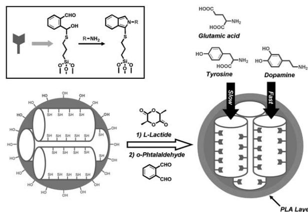
**Fig. 2** Schematic representation of the synthesis of a PLA-coated fluorescent sensor material for the detection of amine-containing neurotransmitters (dopamine, glutamic acid and tyrosine). Box: A fluorescent isoindole moiety is formed in the signalling reaction.
