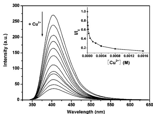
**Fig. 5** Fluorescence changes of a hybrid SBA-based sensor material as a function of increasing  $\text{Cu}^{2+}$  concentration in water at pH 6.0. Inset: titration curve. (Reproduced with permission from ref. 33. Copyright Royal Society of Chemistry.)
