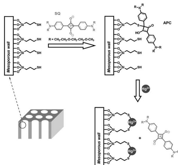
**Fig. 7** Hybrid system with sensing and sorption functions for  $\text{Hg}^{2+}$ .
