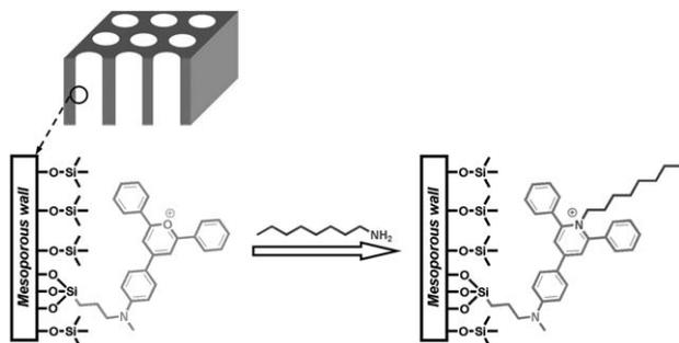
**Fig. 3** Schematic model of a biomimetic hybrid for amine signalling. Changes in colour are due to the reaction between the pyrylium ring and the primary amine. Short amines are too hydrophilic to enter and long-chain amines clog in the pore openings.
