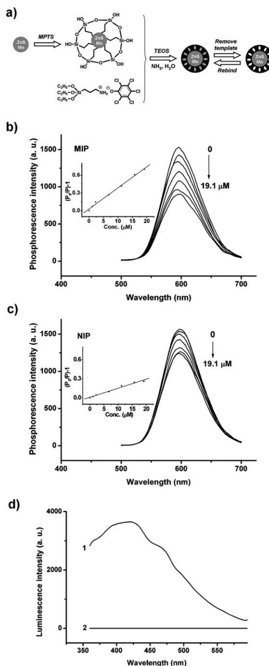
**Fig. 13** a) Schematic illustration for the fabrication of MIP-capped Mn-doped ZnS QDs; RTP emission spectra of (b) MIP- and (c) NIP-capped QDs after addition of the indicated concentrations of PCP in pH 5 acetate buffer; (d) fluorescence (curve 1) and RTP (curve 2) spectra of a real water sample. (Reproduced in part with permission from ref. 64. Copyright American Chemical Society.)
