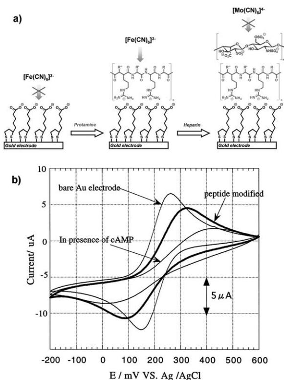
**Fig. 14** a) Architectures of ion channel sensor materials for protamine and heparin detection; (b) cyclic voltammograms of the ferrocyanide/ferricyanide redox couple with a peptide-modified gold electrode in the absence and presence of cAMP in Tris-HCl buffer at pH 7.4. (Reproduced in part with permission from ref. 89. Copyright American Chemical Society.)
