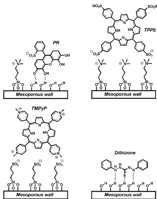
**Fig. 6** Nanocaged monoliths containing selected dyes for the colorimetric signalling of various metal ions.
