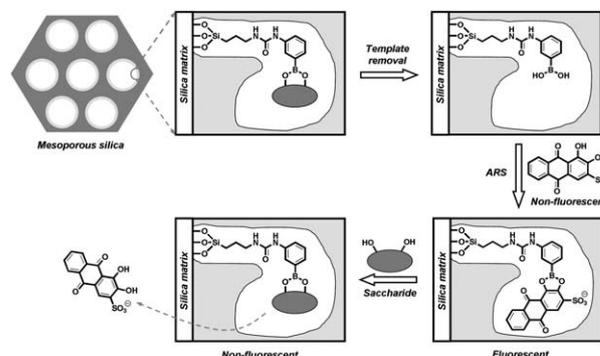
**Fig. 12** Schematic representation of molecularly imprinted mesoporous silica as an indicator-displacement sensor for saccharides.
